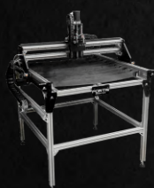
1000 x 1000mm Machine Table
